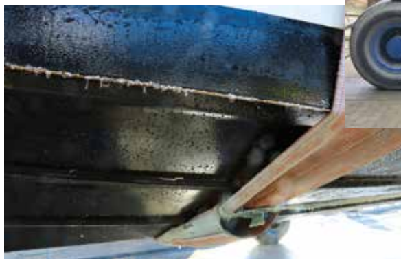
ABOVE After 15 months in the water the Silic One coated hull looks remarkably clean but the untreated drive and trim tabs are heavily fouled LEFT A quick spray down to remove the slime and Fino's hull looks ready for a third season. Note how the water beads on the hydrogel surface
