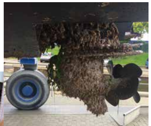
ABOVE After 15 months in the water the Silic One coated hull looks remarkably clean but the untreated drive and trim tabs are heavily fouled LEFT A quick spray down to remove the slime and Fino's hull looks ready for a third season. Note how the water beads on the hydrogel surface
